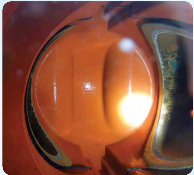
An under-pressure look of clean valve seat.
